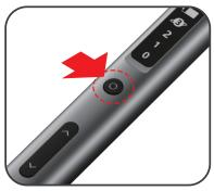
2. Press" **O**", each pres will adjust to a differe gear torque.
