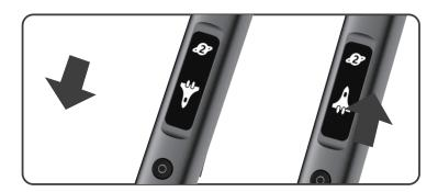
The screen icon shows " A " for twisting the screws tightly, the screen icon shows " W " for twisting the screws loosely.
