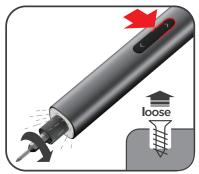
3. Press "^", loosen th screws and turn on th light at the same time
