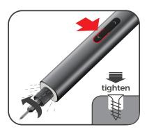
2. Press "\screw", tighten the screw and turn on the light at the same time.
