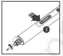
2. Press 3, tighten the screw and turn on the light at the same time.
