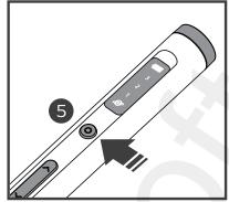
2. Press 5, each press will adjust to a different torque gear.
